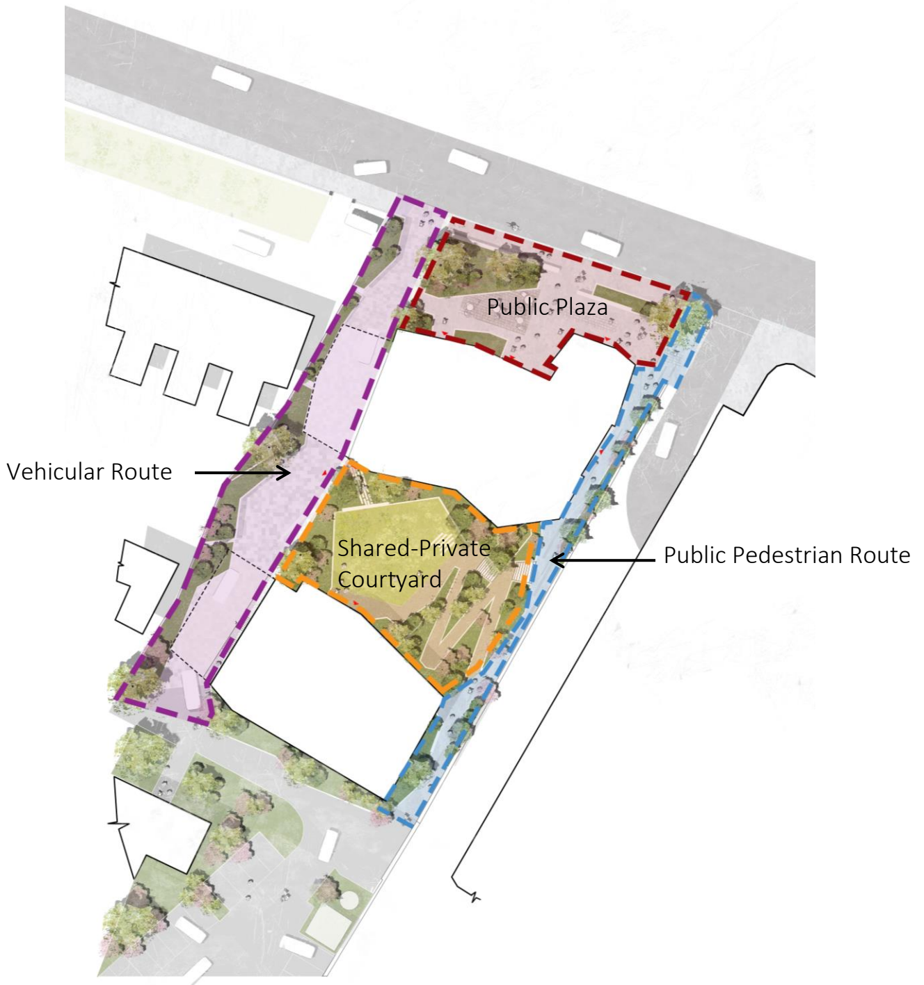
Figure 4: Landscape plan showing the early stages of the design development in particular the extent of the proposed development, public open space and shared-private courtyard at ground level.
